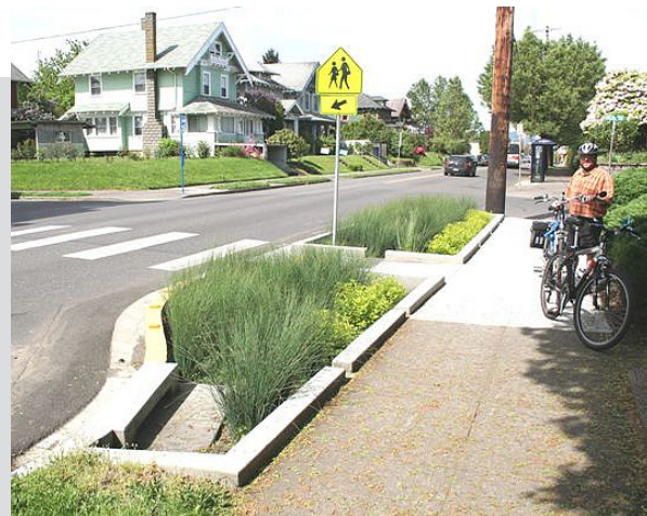
Figures 4-3 & 4-4: Bioswales to remove silt and pollution from stormwater runoff integrated as a landscape feature on a residential street.
