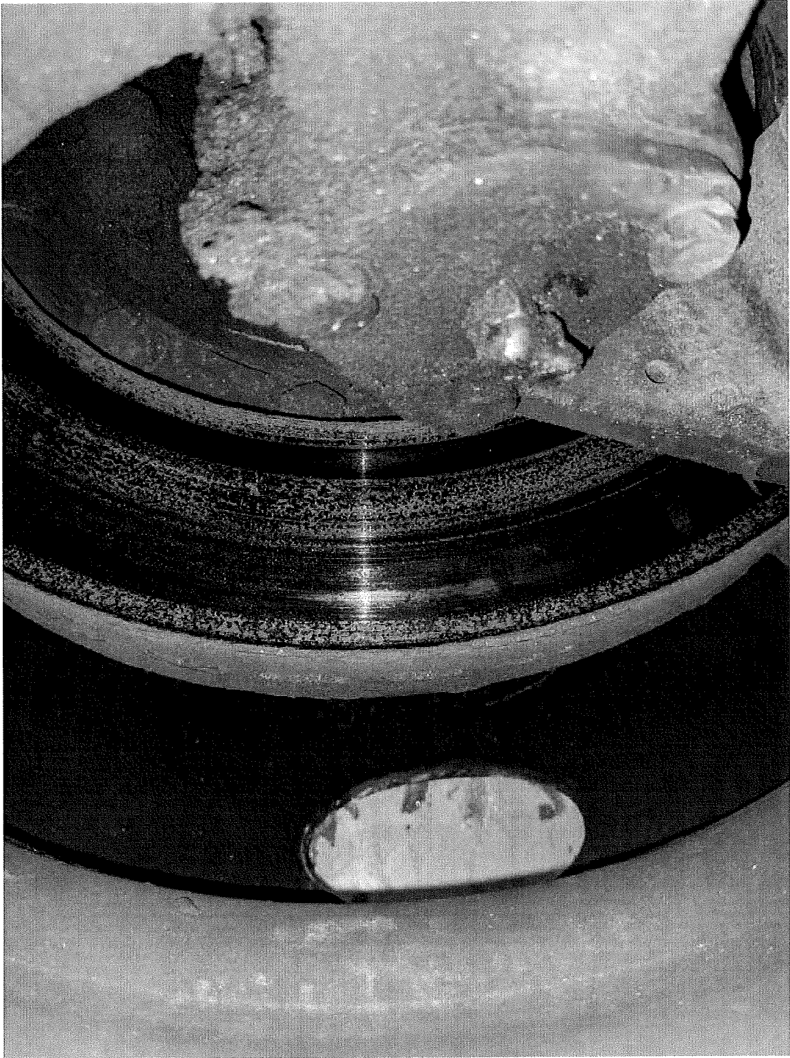
Figure 4- front rotors in need of replacement
