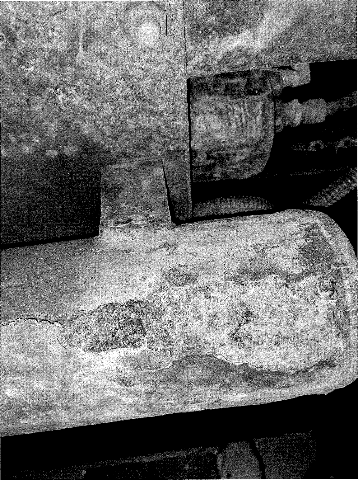
Figure 7- rotting quick recovery tanks
